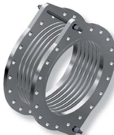
Type 262 is a multi-layer vibration absorber with loose flanges. This expansion joint has tie rods. It is designed specifically to reduce vibrations in the system and noise.
